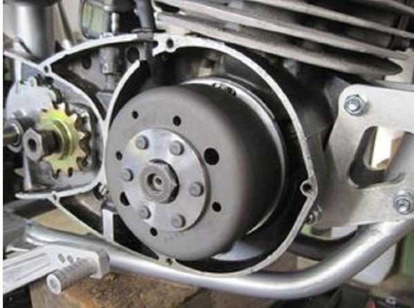
Finally, fasten the rotor carefully with the provided new nut (left-hand thread). Don't forget to use the original washer!
