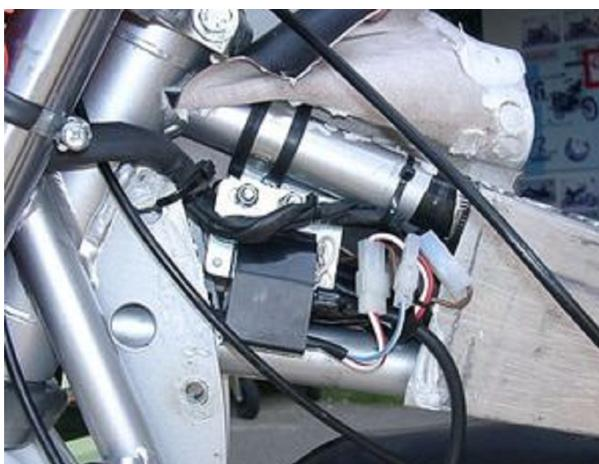
Fasten the ignition coil at a convenient place, favourably near to the spark plug.
