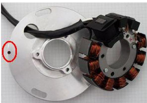
Have a look at the new stator unit. You will find there a small red ignition marking for timing (in the picture a dot, now a line).
