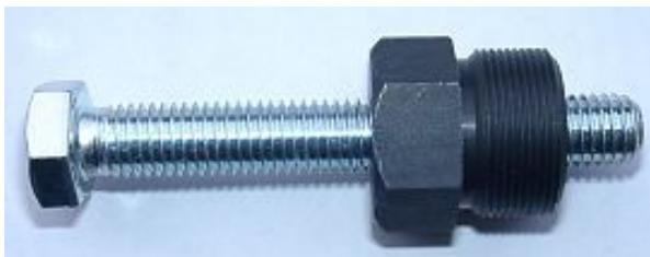
To disengage the new rotor again, you need a puller M27x1,25 (part-no.: 99 99 799 00 **-Not provided!-**).
