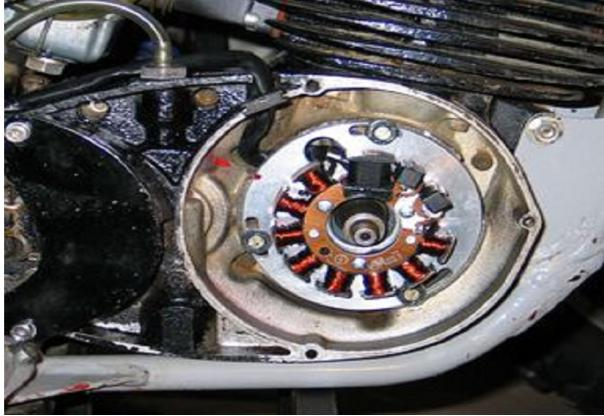
Put the base plate with the stator hanging loosely from the unit into the place of your old generator. Fasten the plate with the 3 screws M5. Take care to not jam any wires under the plate.
