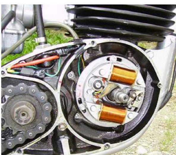
Disengage all wires of the stock FEMSA and ignition coil and take these parts off.
